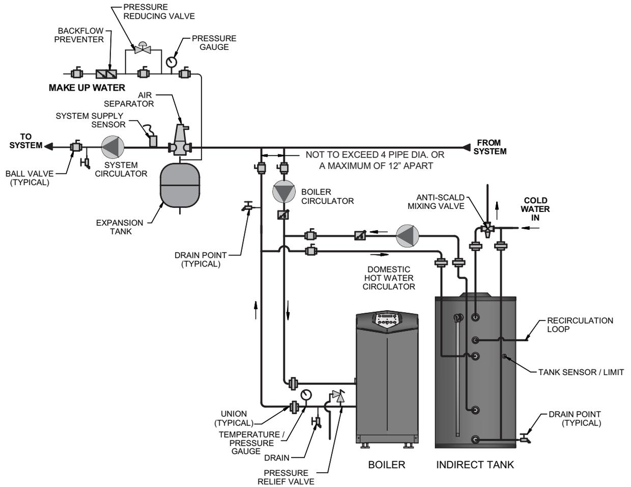
Figure 3-4 Multiple Tank Connections
